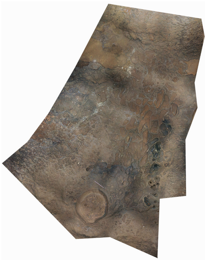
Fig. 15.10 Orthophotography of sector E generated from the photogrammetric survey
