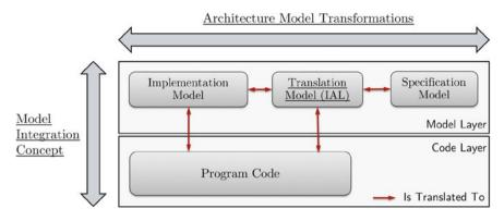
Fig. 1 The view types of the EIA approach and the means to translate between them (underlined)
