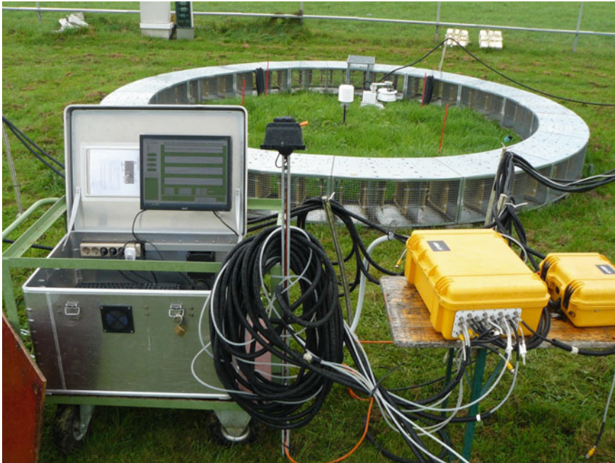
Plate 3.10 The combined automatic chamber system with CRDS analyser for field GHG-flux measurement in the Giessen climate change experiment combining air Temperature warming of +2 °C and free-air CO 2 Enrichment of +20% (T-FACE). In the left-hand box, the Picarro analyser is installed including its monitor and pump. The LI-8150 Multiplexer (big yellow box) is connected to seven automated chambers and eight soil air probes and switches every 5 to 30 min from one port to the next controlled by the LI-8100A Analyzer Control Unit (small yellow box). The screen (lower left side) shows stable N 2 O concentrations (zero flux, 1st panel above), CH 4 uptake (2nd panel), stable H 2 O concentrations (3rd panel), and ecosystem CO 2 respiration (4th panel on the screen)
