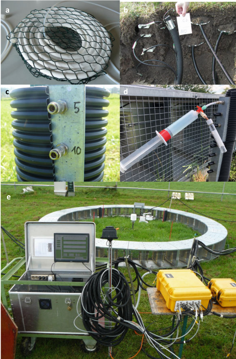
Plate 2.13 Air sampler setup using Accurel ® tubing with a soil air sampler with in- and outlet to allow continuous analysis, note the chicken wire around the sampler is there to protect the material from rodent bites, b soil profile setup with soil air samplers (right) and soil moisture/temperature sensors (on left) which are connected to a datalogger, c manifold system with quick connector gas sampling ports for different depths, d discrete sampling with a syringe and an exetainer vial, first the sample will be taken by the syringe and then the three-way-tap will be turned towards the evacuated exetainer and the gas in the syringe will be transferred to the vial, e the manifold can also directly be connected to an autoanalyzer arrangement for automated in situ measurements (see also Sect. 3.2.2 for further information)
