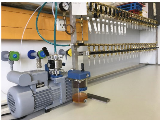
Plate 2.6 A high-efficiency vacuum pump connected to a system for simultaneous evacuation of multiple gas vials
