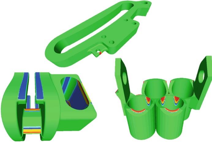
Fig. 6. Example 3D models with colorization of thin areas. Red areas are beneath a threshold value of 0.5 mm.
