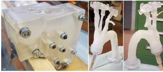
Fig. 10. Casting mould (Clear Resin) for the creation of the wax model (a), the assembled wax model with attached adapters/Elastic Resin) (b), application of the silicone layers (c)
