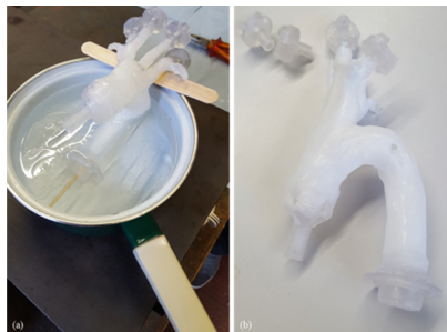
Fig. 11. Melting of the wax in a water bath (a), silicone model after loss of wax with detached adapters and wax layer outside and inside (b)
