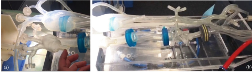
Fig. 14. Geometric comparison of the aorta model from United Biologics (above) with the aorta model made of Elastic Resin, manufactured on Formlabs Form 3 (below). (a) Comparison of the aortic arch with outlets, (b) comparison of the remaining aorta
