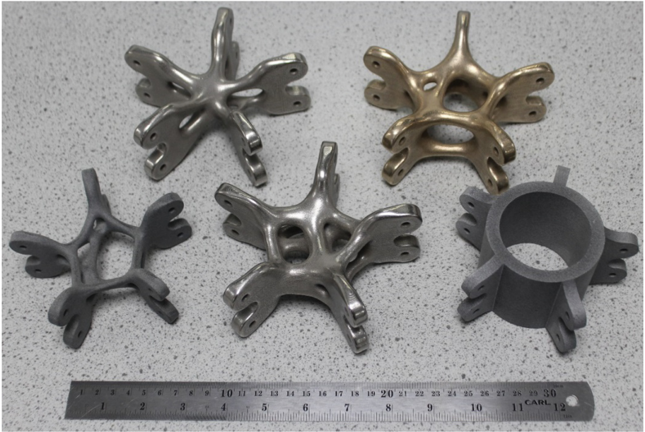
Fig. 18. Additively manufactured node-connection designs.
