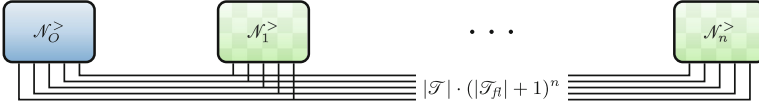
Fig. 4. Overview of the parallel approach : The n subnets are connected such that for every transition t \in \mathcal{T} there are (|\mathcal{T}(t)| + 1)^n transitions, i.e., there is one transition for every combination of which transit of t (or none) is tracked by which subnet. We use until operators in the constructed LTL formula to only skip steps not involving the tracking of the guessed chain in the flow formula.
