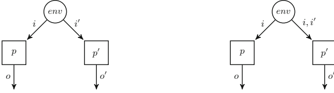
(a) Information fork: An architecture with two processes; process p produces output o from input i and p' produces output o' from input i' . (b) No information fork: The same architecture as on the left, where the inputs of process p' are changed to i and i' .
