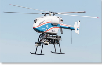
Fig. 1. DLR’s autonomous superAR-TIS equipped with optical navigation.
