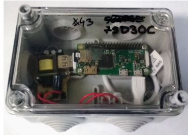
Fig. 3. The Hub in IP57 enclosure
