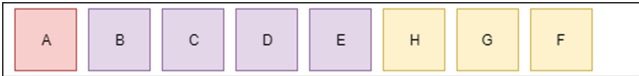
Fig. 5. The run of a breadth-first search with respect to A as the starting node
