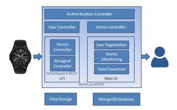
Fig. 4. Biosignal Collection server architecture.
