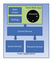
Fig. 2. Smartwatch application architecture.
