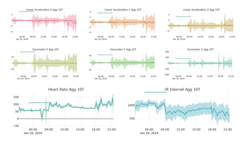
Fig. 6. Visualization of user movement and heart rate data, i.e., accelaration data (top row), gyroscope data (middle row) for all three axis (x, y, z-axis) and data collected by the heart rate monitor (i.e., heart rate and RR-interval data). (Color figure online)
