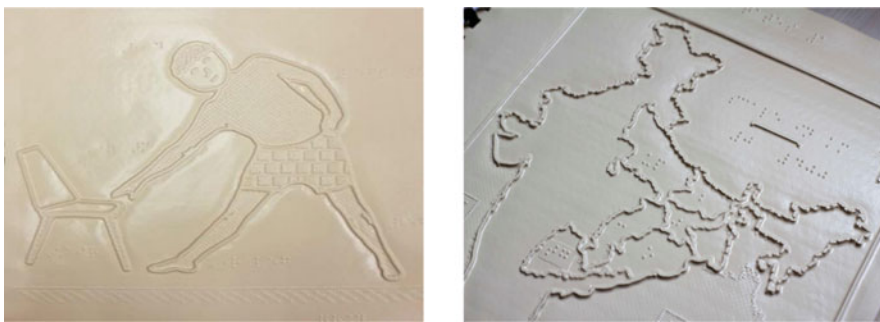
Fig. 5.12 Tactile diagrams developed as part of the project Tactile Graphics sponsored by MEITY, Govt of India made innovative use of 3-D printing for production of low-cost tactile diagrams
