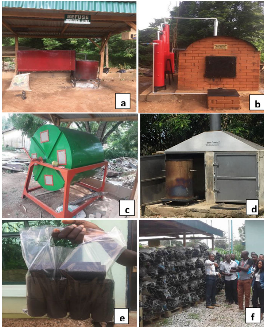
Fig. 5 Other climate change adaptive technologies at RRC: (a) RDF plant; (b) smoke-free incinerator; (c) household composter; (d) smokeless charcoal kiln; (e) smokeless charcoal pellets; (f) wood charcoal
