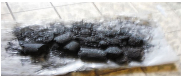
Fig. 4 Bio-char from pyrolysis of woody biomass
