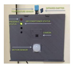
Fig. 2. Hardware device deployed in a room.
