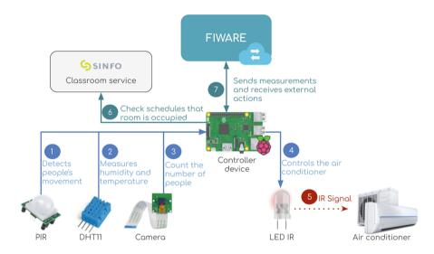
Fig. 3. Hardware measurement and actuation flow.
