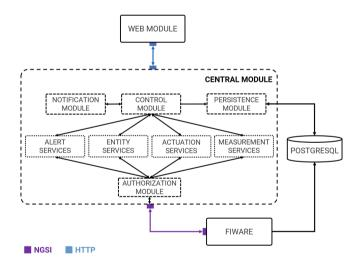
Fig. 6. Internal architecture of Smart Place Web component.
