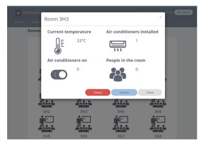
Fig. 7. Visualization of Room 3H3 through the interface provided by the Web module.
