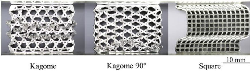
Fig. 12.15 Deformation patterns of Kagome (deformation in X1 -direction), Kagome 90^\circ (deformation in X2 -direction) and square-celled structures at engineering strains of 25% for IP mode and quasi-static strain rates according to [66]
