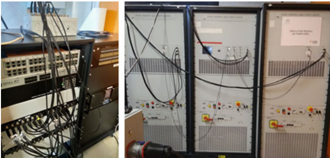
Fig. 14 The RT simulator OP5700 and the Puissance+ Power Amplifier used in the PHIL interface
