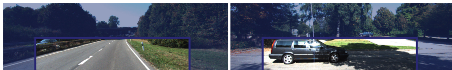
Fig. 5. Images from the KITTI Visual Odometry/SLAM benchmark, Sequence 01 (left) and 03 (right). Since the algorithm is homography-based the images are cropped a priori in order to contain a significant portion of planar or near planar surface. Such an assumption is not valid on all sequences of the dataset, however, certain cases, such as the highway of Sequence 01 (left) is a good candidate. There are several examples where occlusions occur, such as the car in Sequence 03 (right). These situations typically occur at crossroads and turns. Image credit: KITTI dataset [9].
