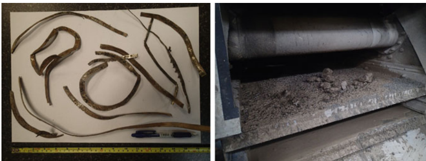
Fig. 7.1 Swarf from a milling operation in the North Sea (Courtesy of equinor)
