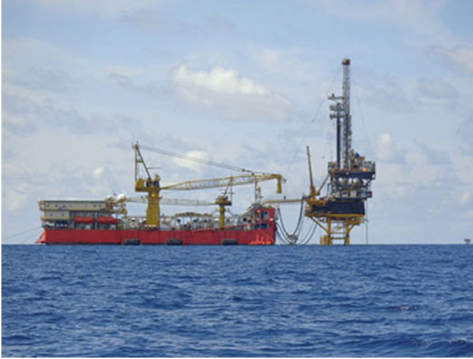
Fig. 5.7 A tender rig in operation while the anchored vessel is in service. (Courtesy of Seadrill)
