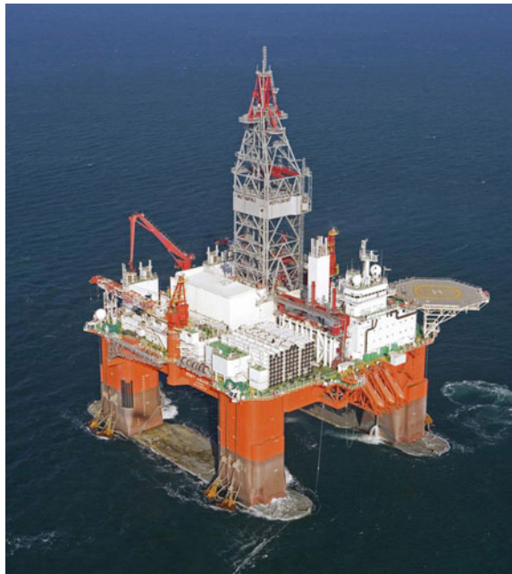
Fig. 5.3 A semisubmersible drilling rig towed to location. (Courtesy of Seadrill)
