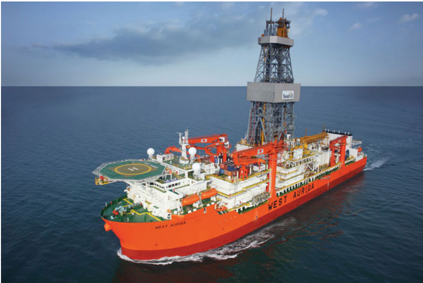
Fig. 5.4 Drillship on location (Courtesy of Seadrill)
