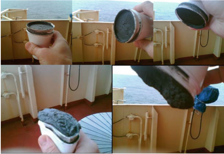
Fig. 4.14 Unconsolidated sand slurry as an alternative plugging material. (Courtesy of FloPetrol Well Barrier)
