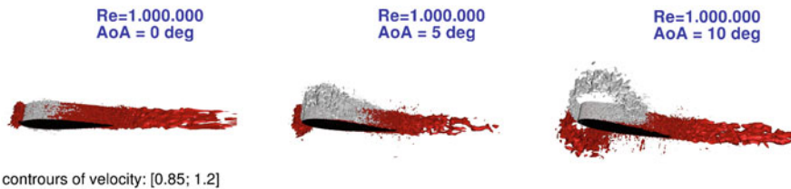
Fig. 2 NACA0012 airfoil at Re = 1 \times 10^6 , from left to right: AoA: 0^\circ , AoA: 5^\circ and AoA: 10^\circ . Simulations are obtained using the incompressible DG solver
