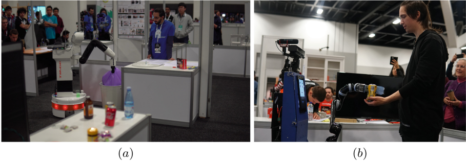
Fig. 7. TIAGo grasping a trash bag during the Take Out The Garbage task using an effort based grasping approach to ensure that the bag was grasped successfully (a) and Lisa handing over a drink to a guest during the Serving Drinks task.
