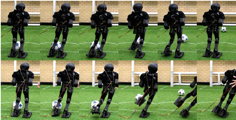
Fig. 3. Time-lapse of two of the kick scripts highlighted in Fig. 2 – Ind_A (top) and Ind_B (bottom) – running on the real NUGus robot. In both cases, the distance travelled by the ball is very similar to the simulated results. However, only for solution Ind_A the robot still stands at the end, while Ind_B leads to the robot falling over – in the simulation, both scripts resulted in the robot standing at the end.
