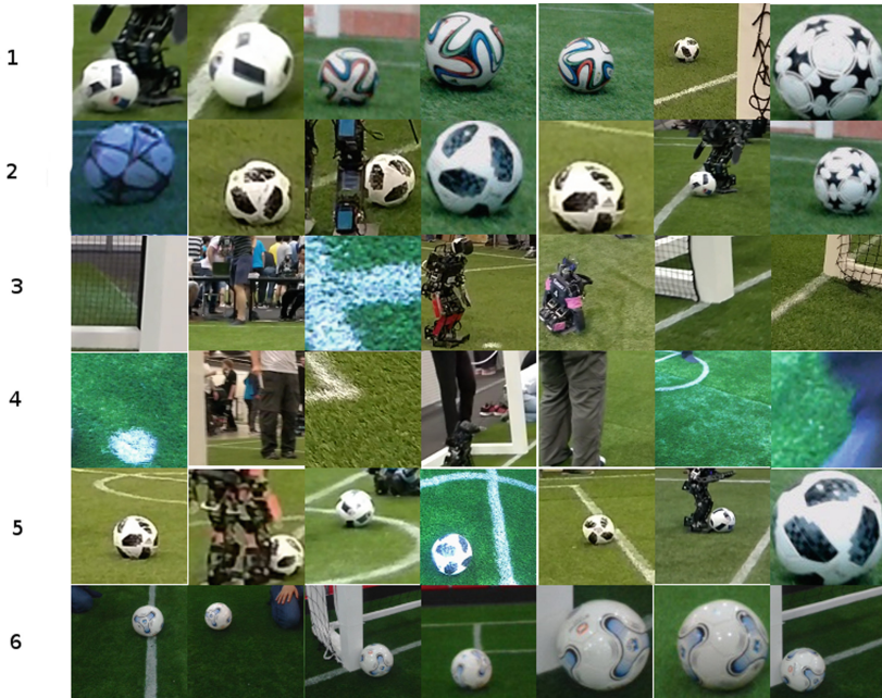
Fig. 3. Row 1, 2: Positive samples in the training data set. Row 3 and 4: Negative samples in the training data set, Row 5: Positive samples of the validation data set. Row 6: Positive samples of generalization data set with a new ball pattern not used for training.
