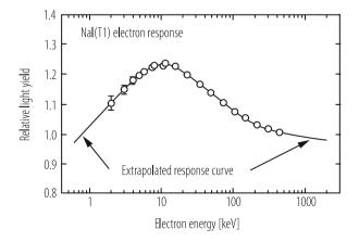
Fig. 3.10 Measured electron response for NaI(Tl) scintillator (from ref [21])
