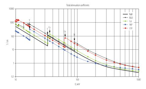
Fig. 3.6 Attenuation coefficients in several high Z materials
