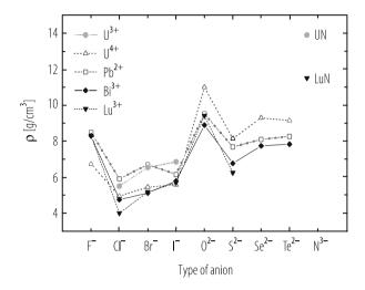
Fig. 3.2 Density for various binary compounds as a function of the binding anion (courtesy P. Derenbos, from ref. [5])
