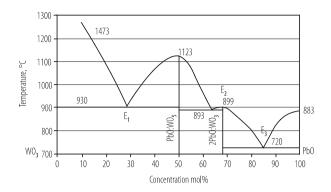
Fig. 3.19 Phase diagram of the PbO-WO<sub>3</sub> system
