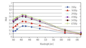
Fig. 3.17 Wavelength dependent absorption coefficient of PWO crystals as a function of the absorbed  $^{60}$ Co dose (courtesy CMS collaboration)
