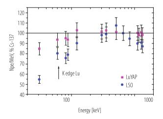
Fig. 3.5 Relative low energy response for LSO and LuYAP crystals, normalized to the <sup>137</sup>Cs energy peak (from ref [13])
