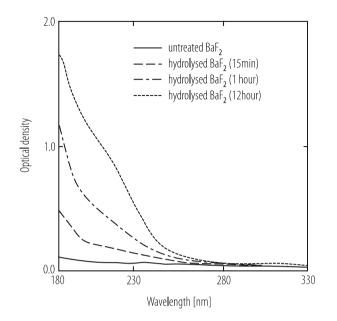
Fig. 3.16 Absorption spectra for different hydrolysed BaF<sub>2</sub> (ref. [28])
