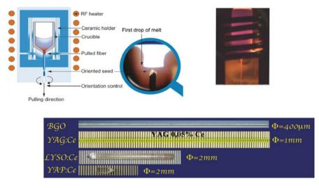
Fig. 3.21 The micro-pulling down crystal growth technology (courtesy Fibercryst)
