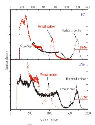
**Fig. 3.13** Energy resolution for <sup>137</sup>Cs photons obtained with  $2 \times 2 \times 10 \text{ mm}^3$  Ce doped LSO and LuYAP crystals measured in horizontal and vertical position. The electronic gain for LuYAP is three times higher to compensate for the lower light yield (6000 pe/MeV and 2000 pe/MeV for LSO and LuYAP, respectively, in horizontal position)
