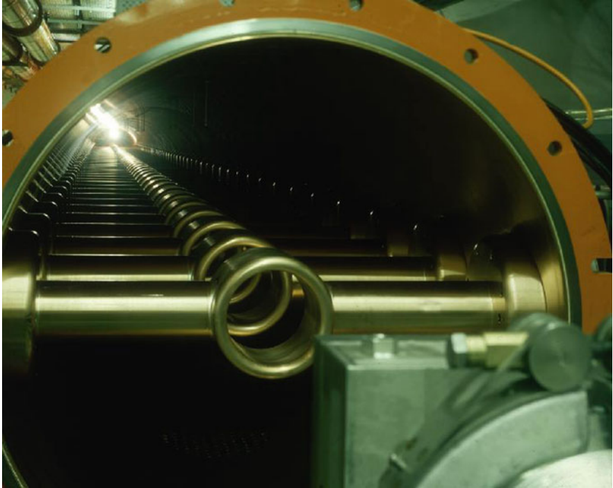
Fig. 8.24 A view inside the CERN SPS 200 MHz travelling wave cavity
