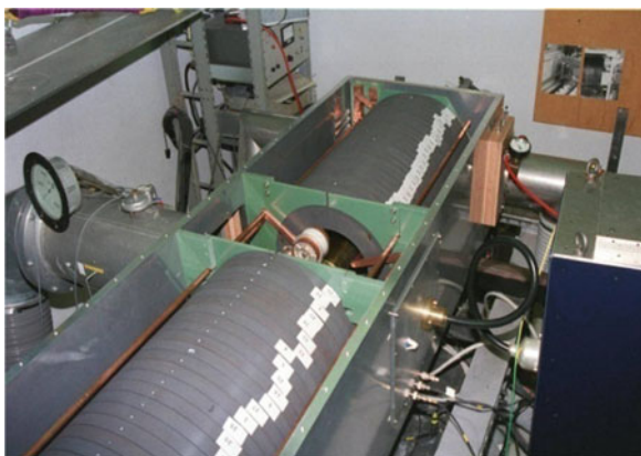
Fig. 8.18 The CERN PSB ferrite cavity with the top cover removed
