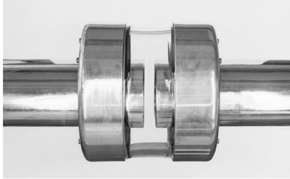
Fig. 8.13 Example of an accelerating gap with glass insulation. It is chosen for illustration; modern insulating gaps use opaque ceramics typically from \text{SiO}_2
