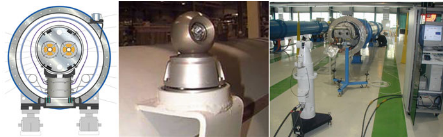
Fig. 8.95 LHC fiducials and fiducialisation equipment
