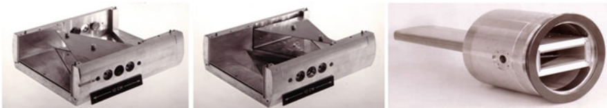
Fig. 8.58 Example of a horizontal shoe box pick-up from the CERN SPS showing right electrode, left electrode and the full assembly in its vacuum chamber
