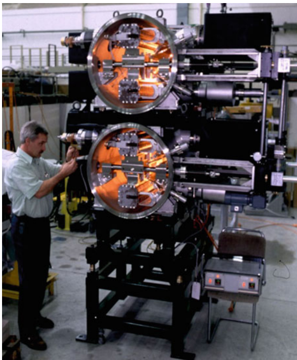
Fig. 8.78 PS Booster extraction septa for the four rings, before closing the vacuum vessels
