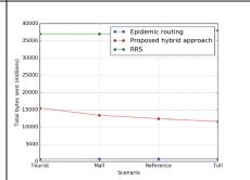
Fig. 2 The new data showing the network overhead for RRS to be much HIGHER than for Epidemic.
