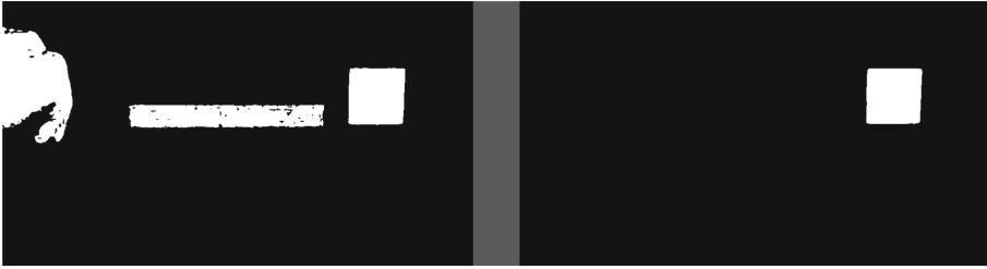
Fig. 3. Identification of red landmarks. Left. Excess red image. Right. Binarized image, threshold = 38. (Color figure online)
