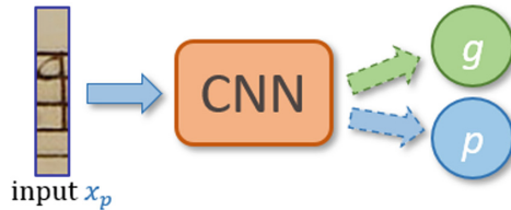
Fig. 7. Multiple outputs model: enlarged images are provided as input and the model must predict both the glyph and the position separately.
