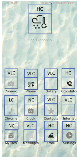
Fig. 3. Example of a synthetic home screen with icons at different levels of contrast and their labels as classified by our tool. Tags: Very Low Contrast (VLC), Low Contrast (LC), Normal Contrast (NC), and High Contrast (HC).
