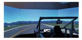
Fig. 1. Fixed-base driving simulator used in the experiment
