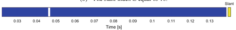
(c) The slant index is equal to 11. One event interval (13 ms) is greater than the others which are all equal to 12 ms.
