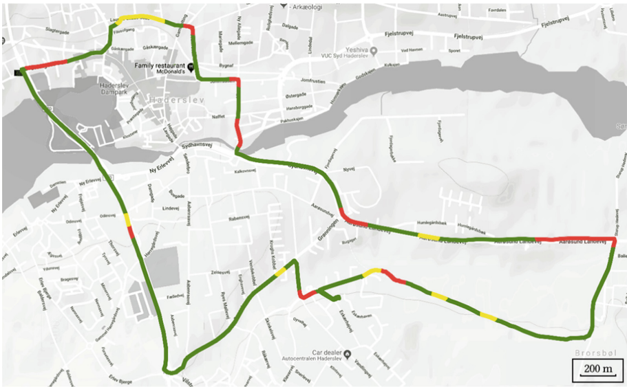
Fig. 2. First route driven by test participant T1, with color coded LowCO 2 (Green), MediumCO 2 (Yellow), and HighCO 2 (Red) peaks. (Color figure online)
