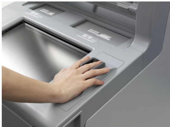
Fig. 6.9 Finger vein device installed on ATM
