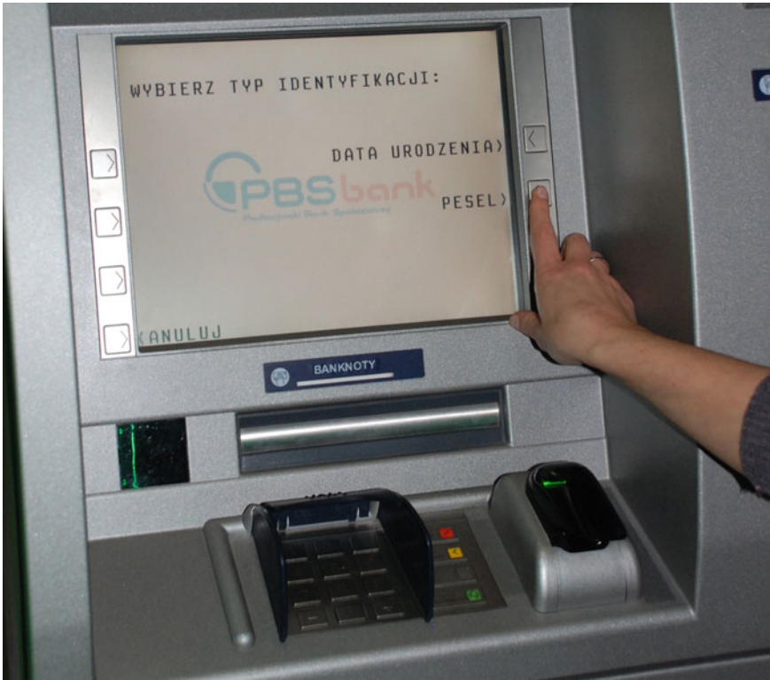
Fig. 6.11 Outdoor ATM finger vein reader installed on an ATM
