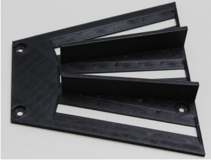
Fig. 3.14 Finger placement unit: the finger-shaped grooves guide the capture subject in placing their fingers correctly. The walls are blocking diffuse emitted light from adjacent fingers, the light transmission illuminators are placed underneath the rectangular holes
