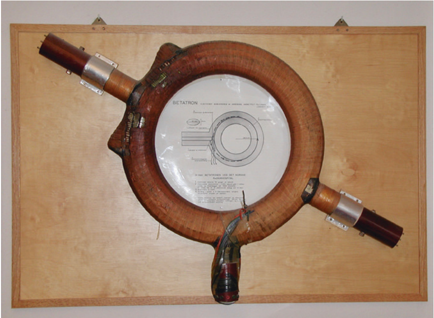
The acceleration tube from the Norwegian Radium Hospital's first betatron, on display in a glass cabinet in the hospital vestibule. (Photo Knut Bjerkan)
