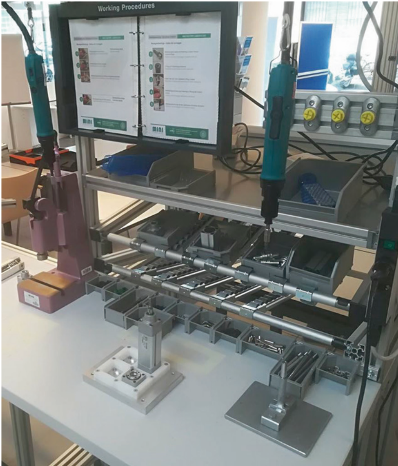
Fig. 12.6 Manual assembly workstation for assembly of pneumatic cylinders (Figs. 12.6–12.11 reproduced with permission from Smart Mini Factory Lab, Unibz)
