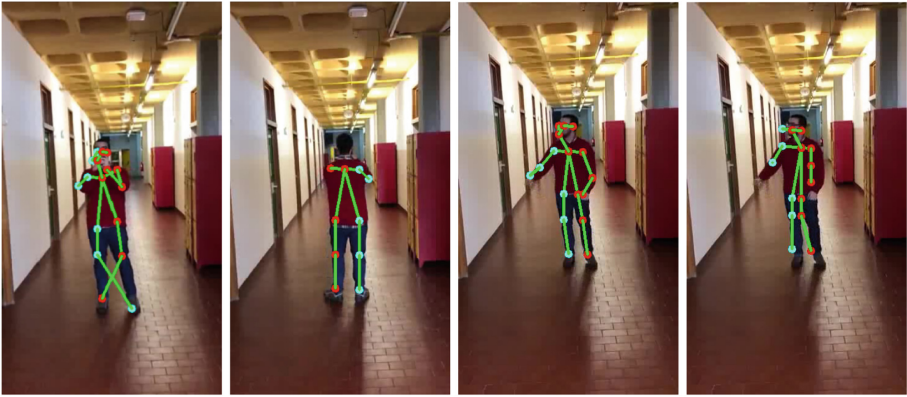
Fig. 4. Left to right, example of confusion between left and right ankle, the correct detected pose, and the pose estimation with spatial size of the CNN equal to 368 \times 368 px and 192 \times 192 px. (Color figure online)
