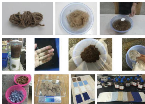
Fig. 2. Paper making process – take the treatment of hemp rope as an example. (Color figure online)
