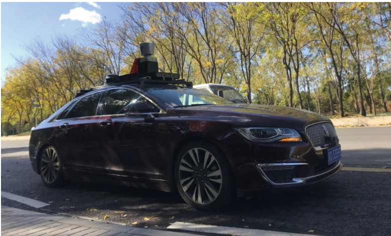
Fig. 2. The prototype of an autonomous vehicle used by passengers for the trial ride (a modified Lincoln MKZ)
