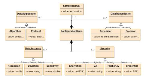
Fig. 5. An example of configuration items (sensing service)
