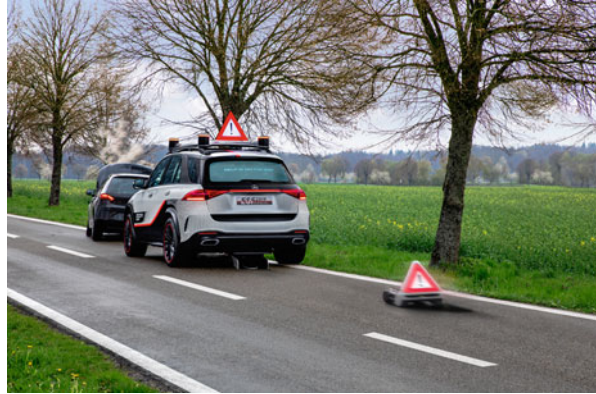
Fig. 17 Securing the scene of an accident – warning triangle robot and roof warning triangle
