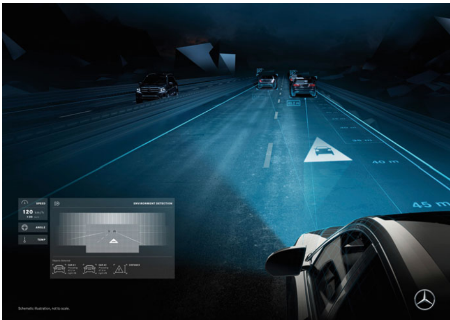
Fig. 8 DIGITAL LIGHT – projection of symbols onto the road in HD quality
