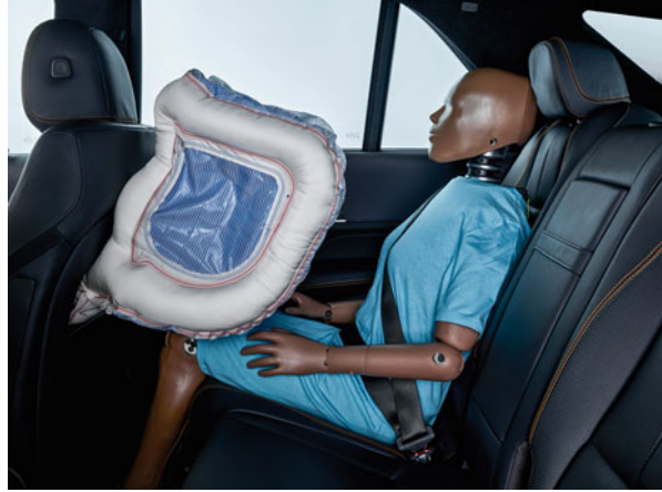
Fig. 16 Rear bag within the seat backrest for a particularly gentle deployment
