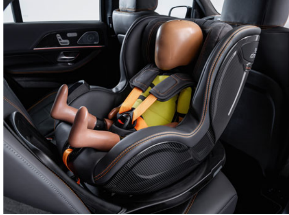
Fig. 9 Networked child seat with PRE-SAFE ® functions
