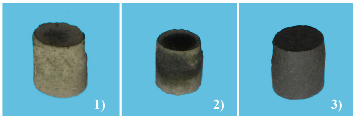
Fig. 1. Appearance of clinker samples produced by separate introduction at burning temperature of: (1) 1250 °C; (2) 1275 °C; (3) 1300 °C.
