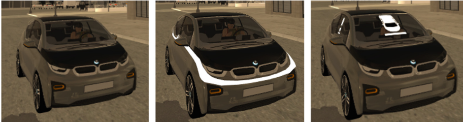
Fig. 1 eHMI Variants used in the study (from left: Baseline, Light-band, Icon)
