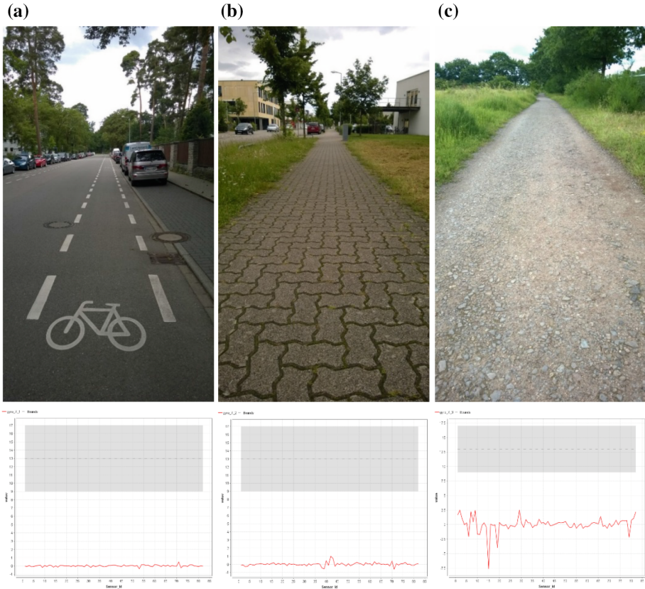
Fig. 10. a. Image and corresponding graph of rotation speeds occurred cycling a cycleway with quality class 1. b. Image and corresponding graph of rotation speeds occurred cycling a cycleway with quality class 2. c. Image and corresponding graph of rotation speeds occurred cycling a cycleway with quality class 3.
