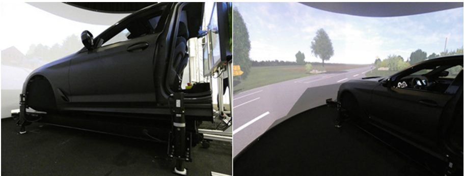
Fig. 2. 3-DOF driving simulator system used in the validation study
