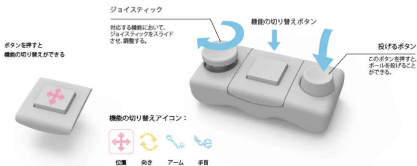
Fig. 3. A prototype combining a joystick and a button
