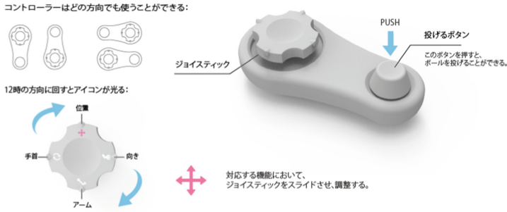
Fig. 4. A prototype combining a rotary selector
